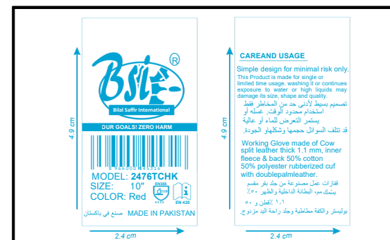
LABEL (WIDTH:2.4CM & LENGTH 4.9CM) (ONLY ON Left SIDE OF GLOVE) (LABEL COLOR :Blue )
